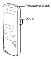
If you connect commercially available headphones to the  $\bigcap$  (headphone) jack before you start, you can monitor the recording. You can adjust the monitoring volume by pressing VOL +/–, but the recording level is fixed.
